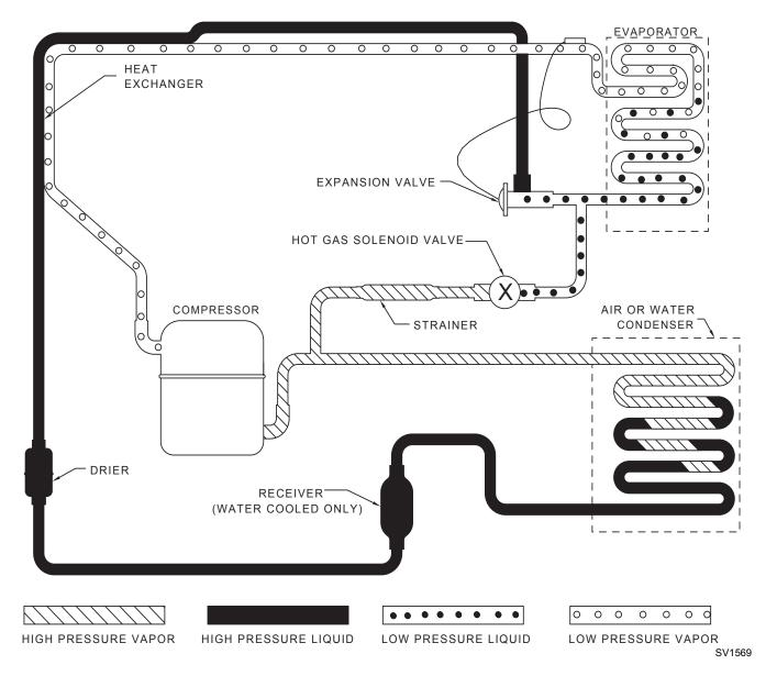
Figure 7-1. Self-Contained Prechill and Freeze Cycle
